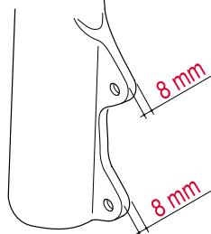
**ATTENTION:** If the thickness of the relative attachment on the fork or frame is less or more than 8mm it will be necessary to substitute the fixing screws with screws of the correct length.
