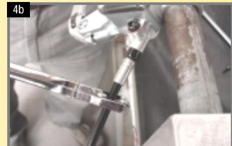
**ATTENTION: Be careful when using the cutter because the blade is extremely sharp and could cause serious injury if not used properly. Do not use blades or saws that could squash or lacerate the tube and therefore could create leakages of brake fluid and therefore an inefficient braking system.**
