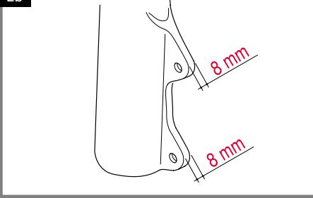
2c: FORMULA supplies appropriate supports to mount between the frame/fork and the brake pincer to adapt the frame/forks to different available brake discs.
