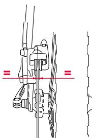
2d: Mount the wheel and fix it with the original fixing nuts, rotate it slowly and check that the disc is centralised between the pads and that no parts come into contact. Effectuate two or three braking actions to bring the pads to the correct distance from the disc.
